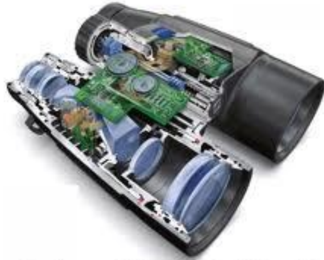
Structura unui binoclu Zeiss Victory RF 8x45
